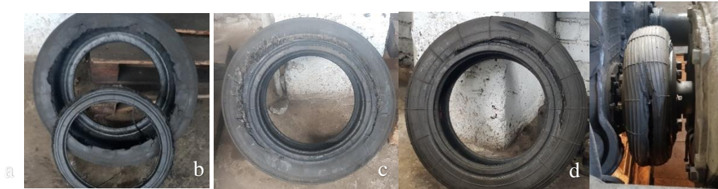
Fig. 2. Types of failures of rubber-cord couplings: a; b; c – rupture of the side surface; d – rupture of the upper surface
