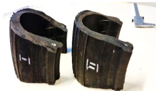
Fig. 5. General view of fragments of rubber-cord couplings
